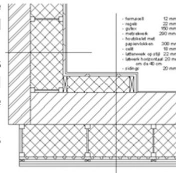
Detail and thermal bridge simulation of the connection between facade and common wall
