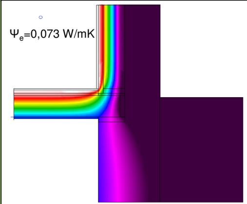
Construction detail and thermal conductivity image of the connection floor slab - façade
